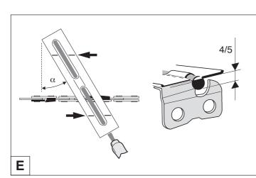
A file holder makes file guidance easier. It is marked for the correct sharpening angle of:
