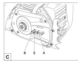
Turn chain tensioning screw (4) to the left (counter-clockwise) until the pin (5) of the chain tensioner is underneath the threaded pin (6).
