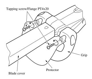
(2) Loosen Pan head screwM5x25s(2pcs) fixing Grip with Housing, and pull out Grip toward the arrow direction, extending it outside a little.
