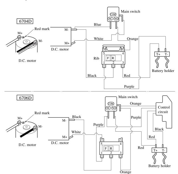
2. Wiring (how to store in Housing) 6704D,6706D < How to store Lead wires>
