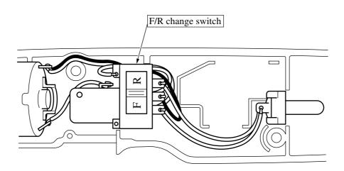
2. Wiring (how to store in Housing) 6704D,6706D
